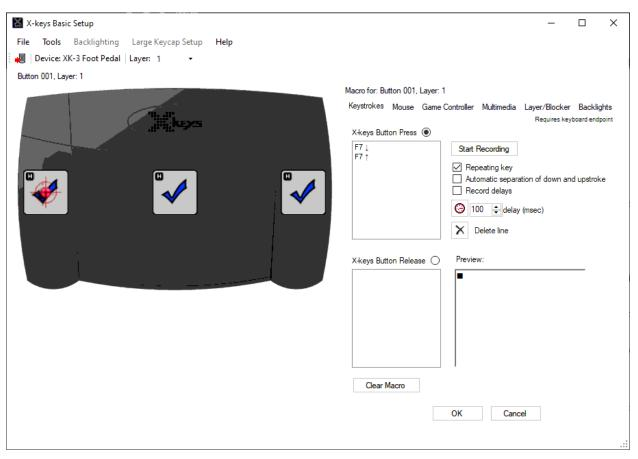
Suggested setup for Rewind. Note the function will 'repeat' when held down, as the "repeating key" option is selected.
