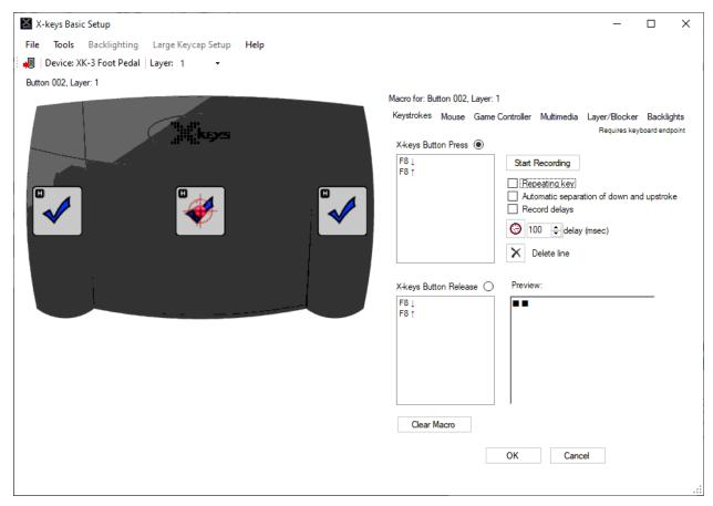
Suggested setup for Play/Pause. This will play the audio while the button is held down, and stop the audio when released. If you would like this function to TOGGLE instead, remove the "X-keys button release" assignments.
